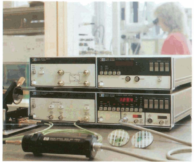
The new optical average power meter features two independent optical inputs and power ratio measurements.
